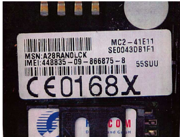
Fig. 2. Label on a European cell phone, underneath the battery. The IMEI number 448835-09-86675-8 is printed on the label and below the numbers is also encoded as a 128 bar code.
